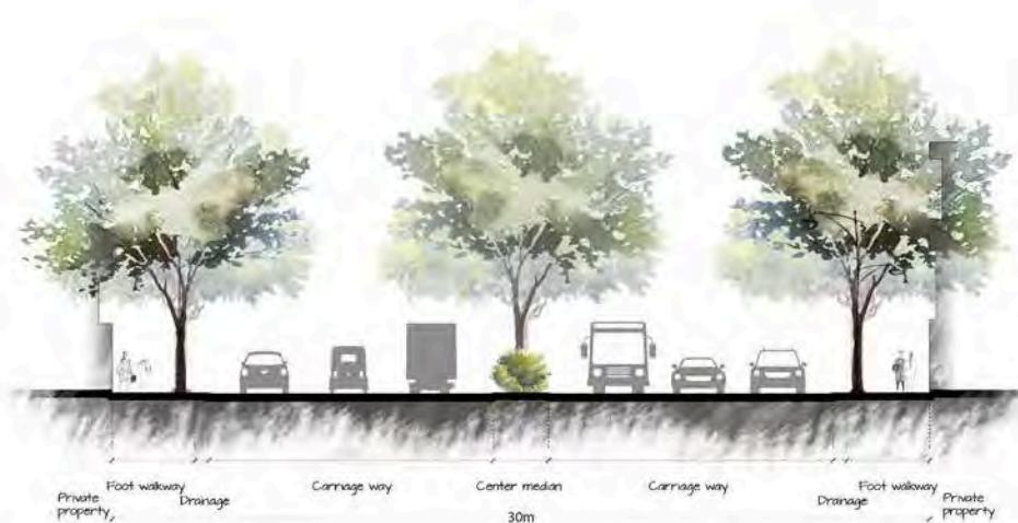
**Figure 5.2:** Recommended typical cross section of P1 road category
