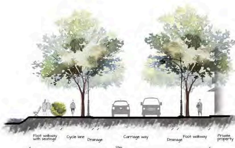
**Figure 5.8:** Recommended typical cross section of P6 road category
