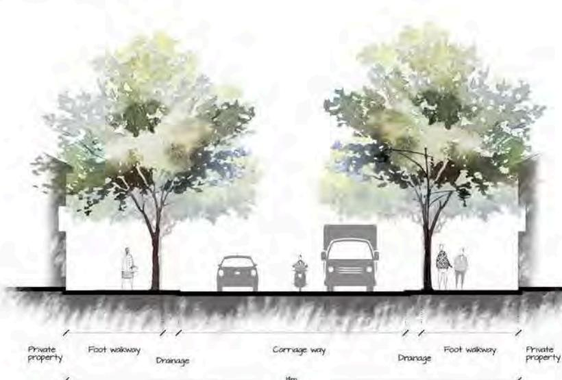
Figure 5.5: Recommended typical cross section of P3 road category
