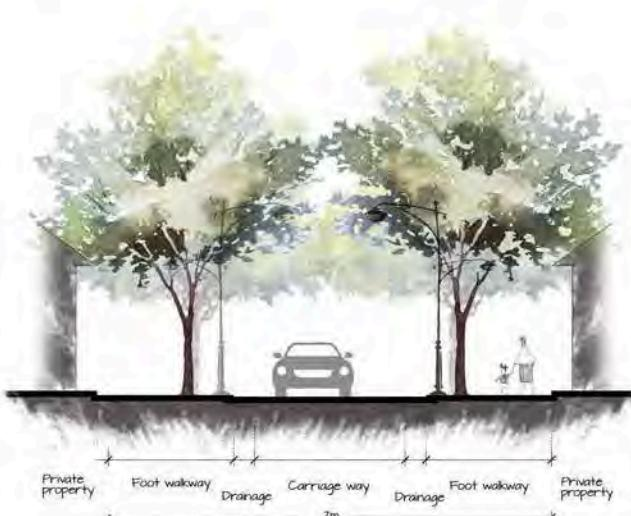
Figure 5.6: Recommended typical cross section of P4 road category
