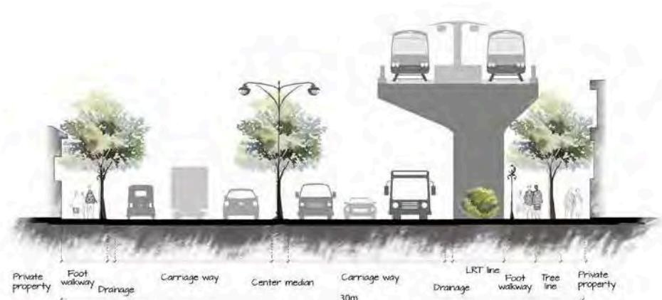
**Figure 5.3:** Recommended typical cross section of P1 road category with LRT
