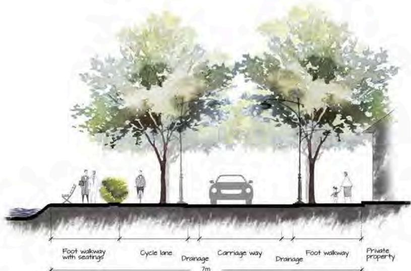
**Figure 5.7:** Recommended typical cross section of P5 road category
